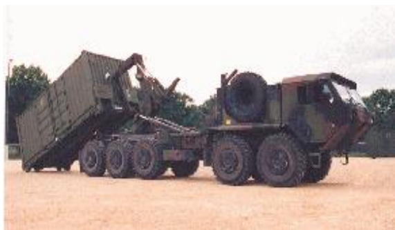
Figure 1. Modular Vehicle with ISO Module and Integral Load Handling System 1
