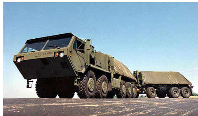
Figure 2. Modular Vehicle with Integral Load Handling System and Modular Trailer both with Flat Rack Modules 2
